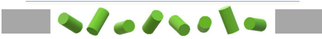
Fig. 1 Schematic cross section of a grid hole with ideally distributed single particles in random orientation
