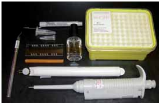
Figure 6: All tools necessary to set up a counter diffusion experiment in CrystalSlide™.
