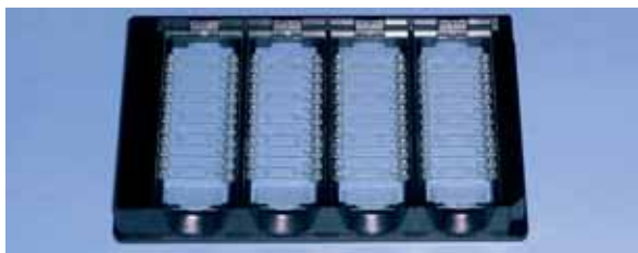
Figure 1: The image shows four CrystalSlides™ in a slide holder.
