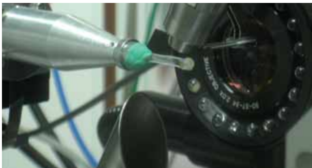
Figure 13: Single channel cut from CrystalSlide™ and mounted in front of an X-ray beam (APS GM/ CA CAT ID-D) for in situ X-ray screening.
