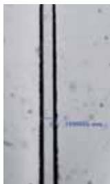
Figure 4: The channel width is 100 µm (ImagePro 6.0).
